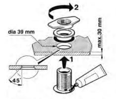
Install flooding valve and sending unit:
