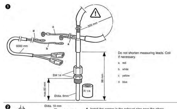
Install the sensor in the exhaust pipe near the elbow flange. Maximum adjustment depth up to the middle of exhaust pipe: 60 mm.
