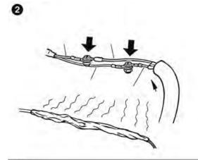
Slide the heat-shrinkable sleeve over the cable connections and then heat with a hot-air fan over the entire length until it shrinks. Always follow the safety advice of the hot-air fan manufacturer.
