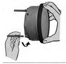
If you would like to omit the fastening nut, you may use the part set A2C59510854 as an alternative. This is recommended if the installation location is subject to vibratory loads.
