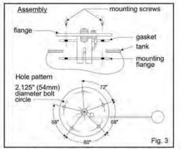
CAUTION: Make certain float arm has a clear field of motion before tightening screws in flange assembly.
