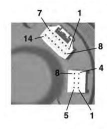
Depending on the configuration, insert the cable into the 8-pin and 14-pin contact housing according to the following pin assignment. The contacts must audibly lock into place.
