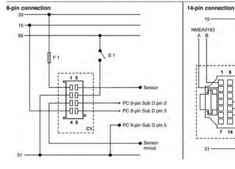
Depending on the configuration, insert the cable into the 8-pin and 14-pin contact housing according to the following pin assignment. The contacts must audibly lock into place.
