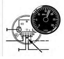
I Select number of cylinders for petrol engines (4-stroke), using a coding switch.
