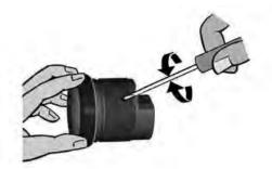
The gauge must be calibrated to the connected immersion tube sensor. Adjust the setting with an insulated screwdriver when the tank is **empty**. Rotate the potentiometer until the gauge reads empty (0 or E).
