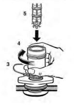
Make a hole 39 mm dia., at a suitable location. The wall thickness can be up to 30 mm. Camber the hole out at 45 degrees for good sealant distribution during the assembly. To install the hull sleeve and the sending unit proceed as follows:
