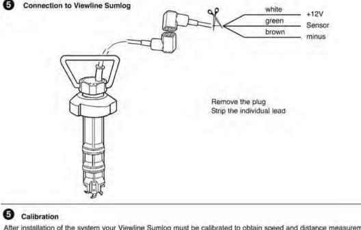
After installation of the system your Viewline Sumlog must be calibrated to obtain speed and distance measurements with the maximum accuracy. FREQUE setting for the die INPUT On the Viewline Sumlog display, select the function.
