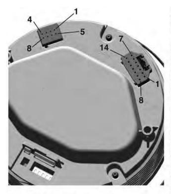
Now insert the plug into the gauge. Note the inverse polarity protection nose in the process. Depending on the configuration, insert the cable into the 8-pin and 14-pin contact housing according to the following pin assignment. The contacts must audibly lock into place.
