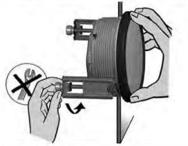
Place the bracket on the stud bolt and hand-tighten the knurled nut.
