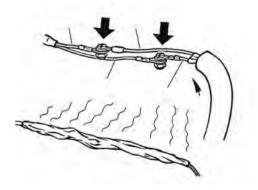
Slide the heat-shrinkable sleeve over the cable connections and then heat with a hot-air fan over the entire length until it shrinks. Always follow the safety advice of the hot-air fan manufacturer.
