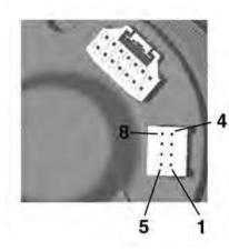
Depending on the configuration, insert the cable into the 8-pin contact housing according to the following pin assignment. The contacts must audibly lock into place.
