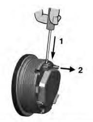
To remove the connector, press the latch (1) and pull the connector out (2).
